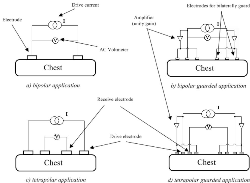
Figure 2. The scheme of the impedance measurement
